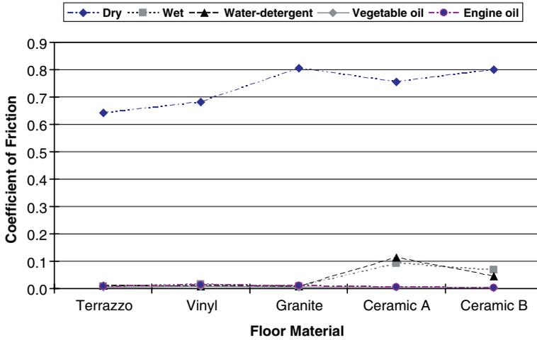
Fig. 3. Interaction between floors and contaminants, the COF values were averaged for footwear materials.
