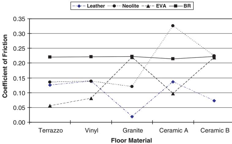
Fig. 4. Interaction between floors and footwear materials, the COF values were averaged for contaminated conditions.
