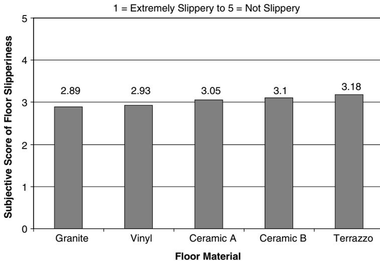
Fig. 7. The effect of floor material on the subjective score of floor slipperiness.
