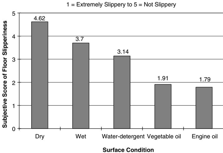
Fig. 6. Subjective score of floor slipperiness under different surface spillage conditions.
