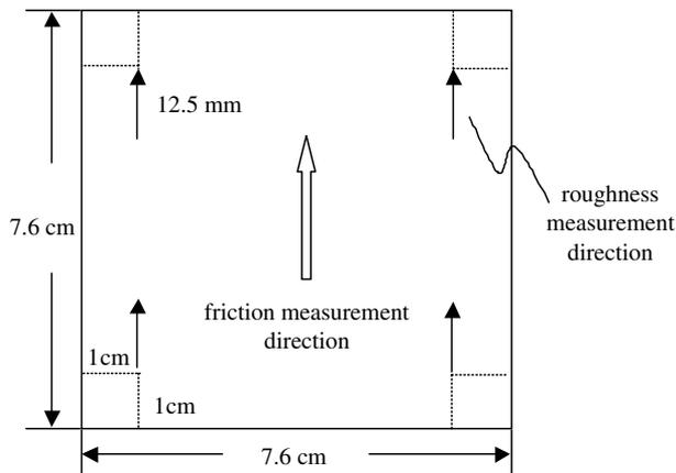
Fig. 2. Locations and direction of friction and roughness measurements.
