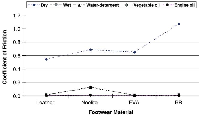
Fig. 5. Interaction between footwear materials and contaminated conditions, the COF values were averaged for floor tiles.
