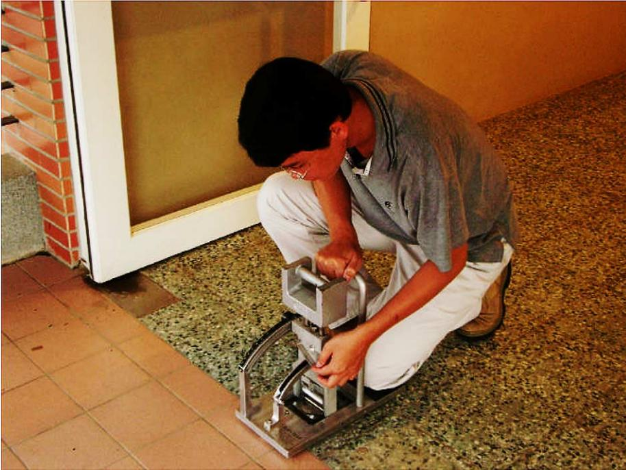
Fig. 1. The Brungraber Mark II used in field measurements.
